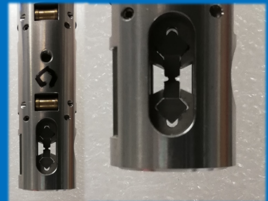
Strain Cell for Applying Uniaxial Pressure
