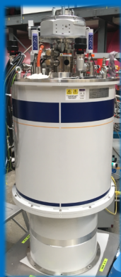
Thermal Expansion Setup for High Magnetic Fields & Ultra-Low Temperatures
