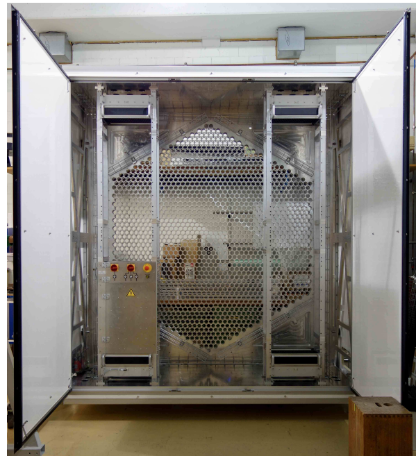
FIG. 6.1 – Assembly work of two prototype camera bodies has started with the aim of shipping the bodies to the integration lab in Heidelberg for the installation of the electronics in summer 2017. Shown is the rear view of one of the prototypes with open doors, installed racks, safety and power cabinet in the left lower corner, as well as the heat exchangers and fan trays.
